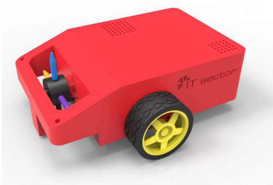
Figure 24: Updated 3D-model Graphbot
